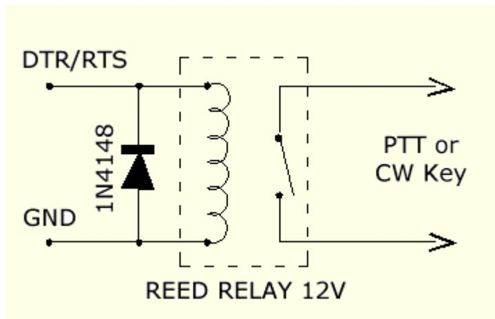
*Serial interface using a reed relay*
