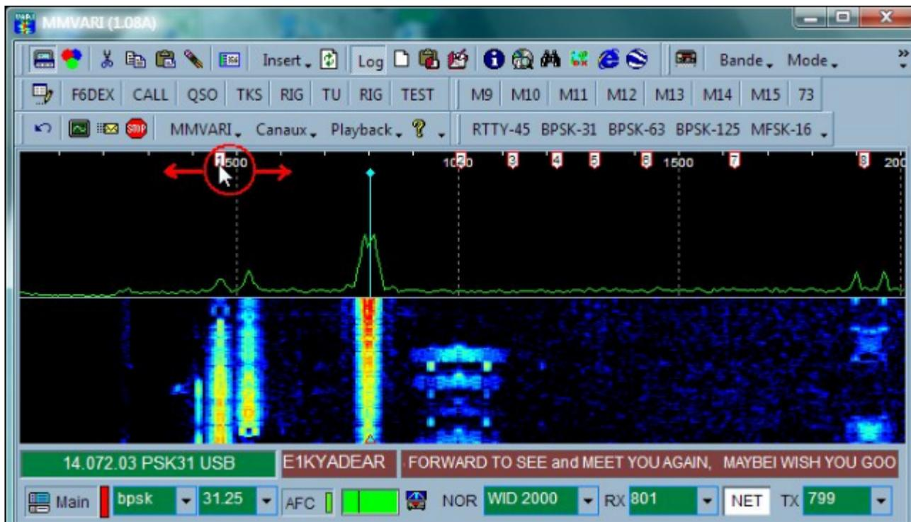
*To set the tone of a sub channel, drag the label or set this channel active and R-Click the waterfall.*
