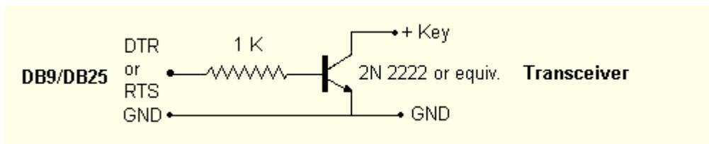
*Serial interface using a transistor (positive keying - not isolated)*
