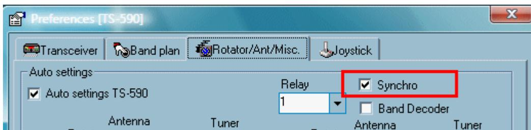
*Synchro option - if required - must be checked for each transceiver (Preferences)*
