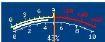
The Bargraph mode features a peak hold function. The maximum s-meter value is displayed and will be reset when beginning a new frequency change or after 2s. An auxiliary bargraph displays the auxiliary meter values.
