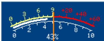
The Analog mode is displayed by default at startup. The linear scale (0-10) displays the auxiliary meter values (see below).
