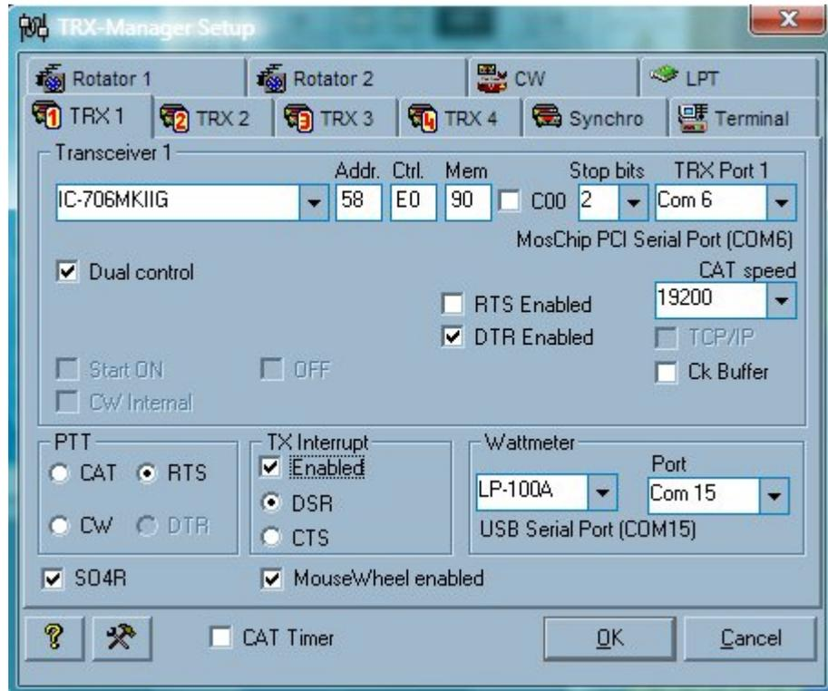
*Interface's RTS line is not used and free for PTT Switching
