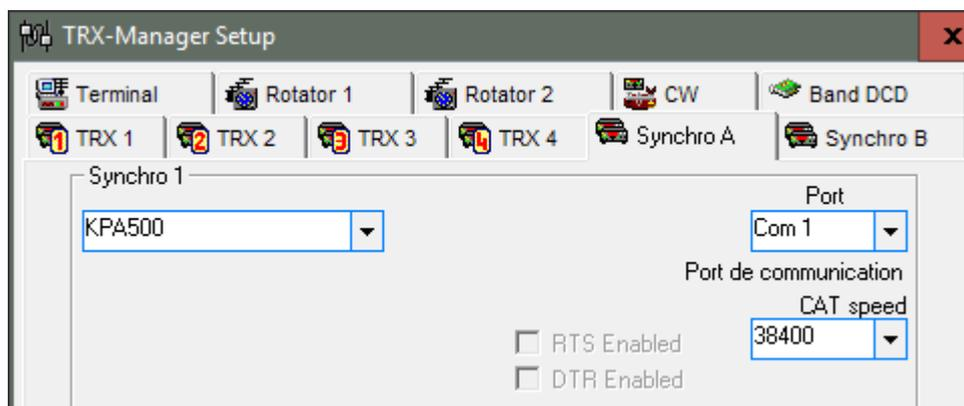
Once configured and restarted, TRX-Manager automatically synchronizes the band switch of the amplifier or the antenna tuner (\*) with your transceiver. In addition, the External menu shows a KPA/KAT500 item which opens a graphical interface to control the most critical functions of the amplifier and/or the antenna tuner.
