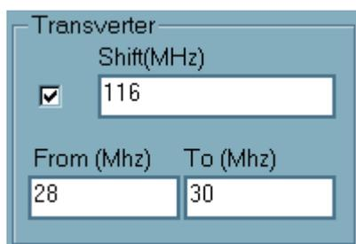
To enable the frequency conversion, you must select (using the program) a frequency within the range of the transverter.
