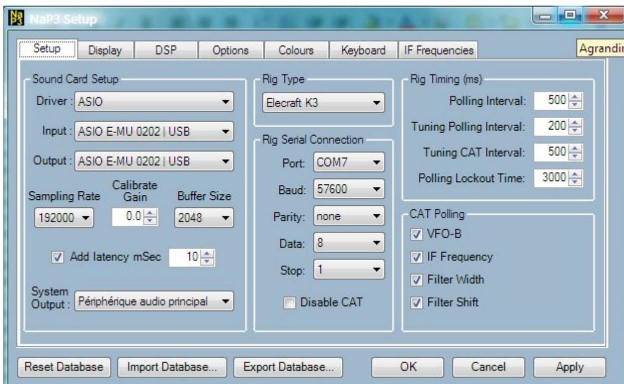
*NaP3 (Setup-IF panel): Note recommended Rig timing with TRX-Manager*
