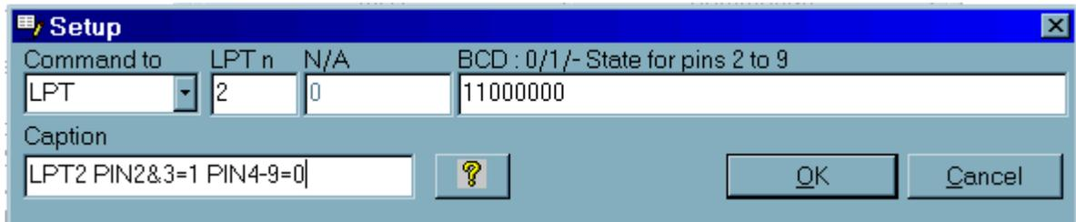
*Setup for LPT2, Pin 2 & 3 = 1, Pin 4 to 9 = 0*
