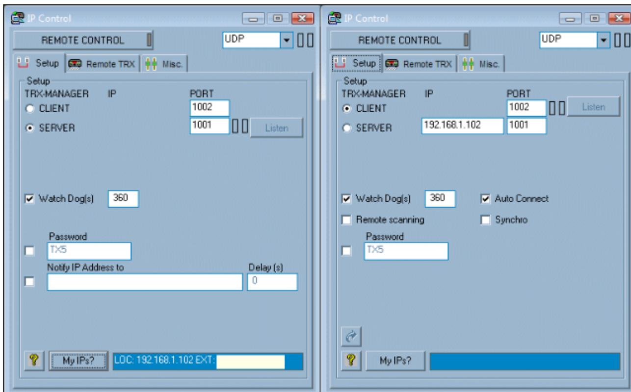
*Typical setup for SERVER and CLIENT using UDP protocol*
